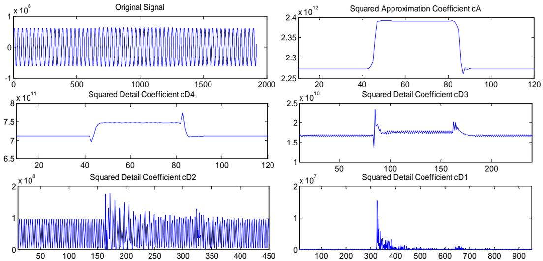
**Figure 4: Squared Wavelet Coefficient of Voltage Signal of Phase-A Using Db4 as Mother Wavelet with Sudden Outage of Load**
