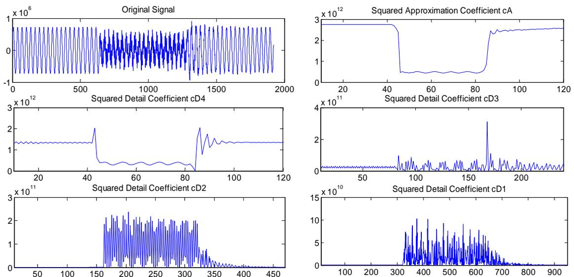
**Figure 8: Squared Wavelet Coefficient of Voltage Signal of Phase-a Using Db4 as Mother Wavelet with Three-phase Fault at Bus-3**
