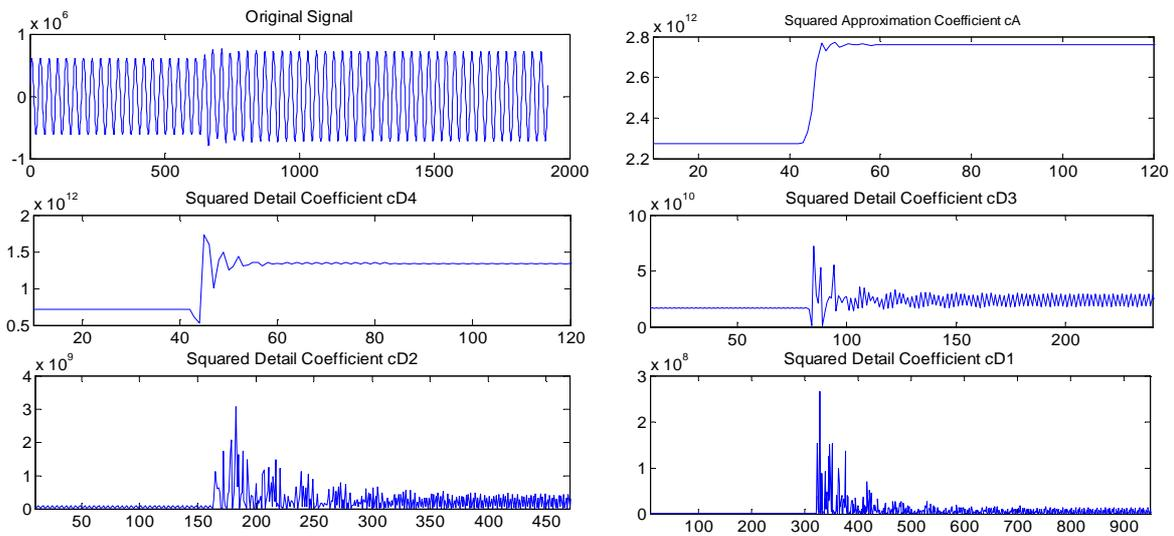
**Figure 6: Squared Wavelet Coefficient of Voltage Signal of Phase-a Using Db4 as Mother Wavelet with Islanding of Test System from Utility Grid**
