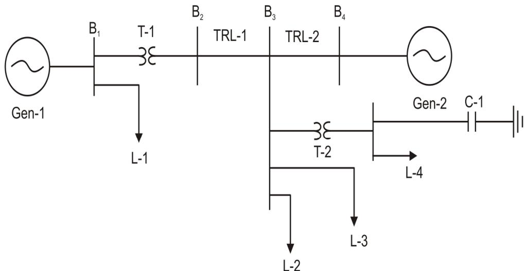
**Figure 3: Proposed Model of Power System for Detection of Disturbances**
